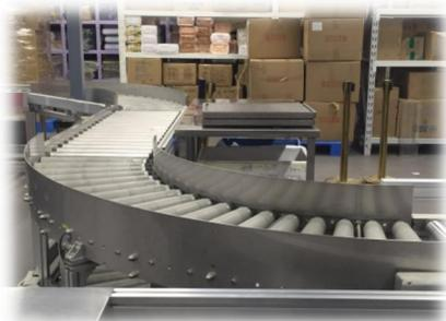
辊筒输送 Sorting device
